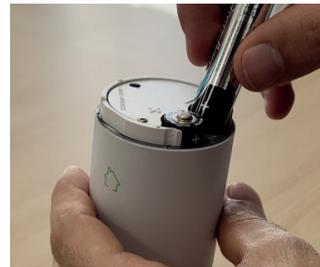
3) Unscrew and remove the TRV+AA valve cover and insert AA batteries, observing polarity.
