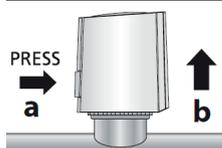
Press the small button on the side of the valve and then lift the body.
